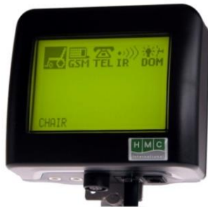
Easy Rider lcd-scherm IR + RF in optie
